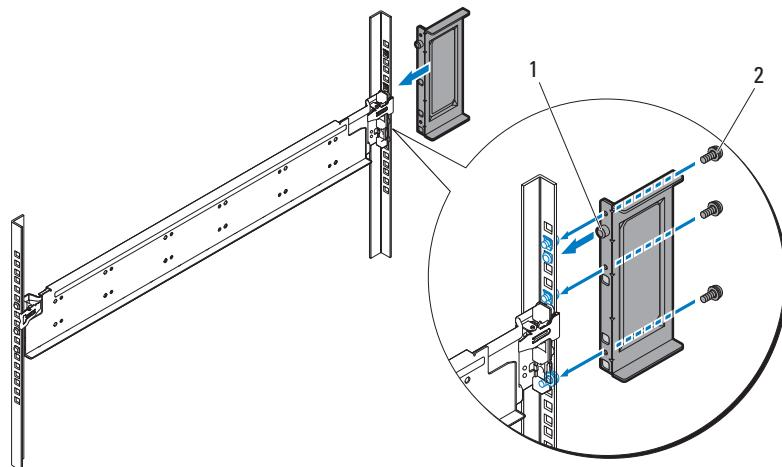
**4 将右导轨和固定支架安装到机架上。**
